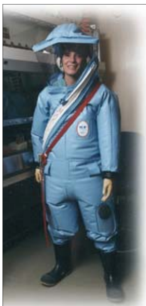
Figure 6. A BSL-4 personnel suit, with air supply provided through the coil coming from the top of the helmet
